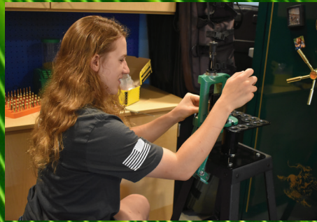
Seating bullets on the RCBS Rock Chucker Supreme Press with a .223 Gold Medal Seating Die.
