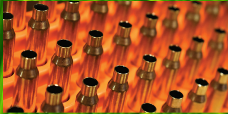
Pre-primed .223 cases prior to being trimmed and chamfered
