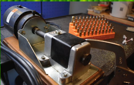
I used a Gracey trimmer to trim and chamfer the cases prior to loading.
