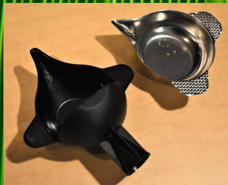
I prefer a powder dish with a funnel (left) to avoid powder spillage.
