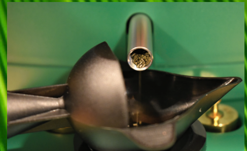
The RCBS Chargemaster Combo would dispense powder automatically when I replaced the powder dish that I had previously zeroed.
