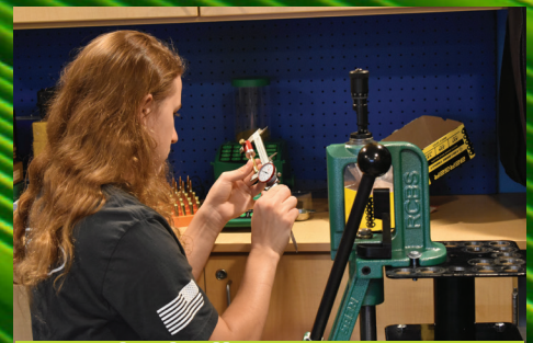
I used a bullet comparator to measure the ogive.
