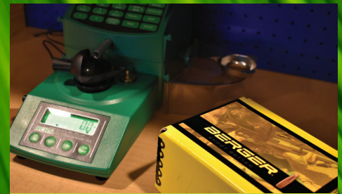
I zeroed the scale with the powder dish before measuring each charge.
